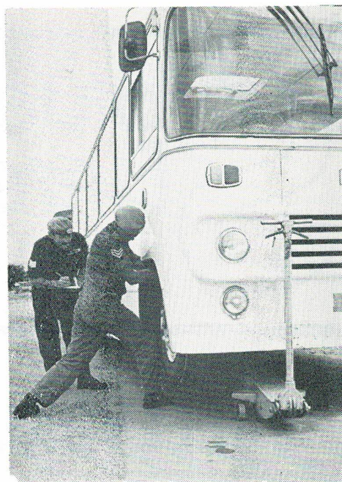
Sgt John Wilkinson and Sgt Alan Clifton carry out an inspection of a UN bus, in this case wheel bearings.
