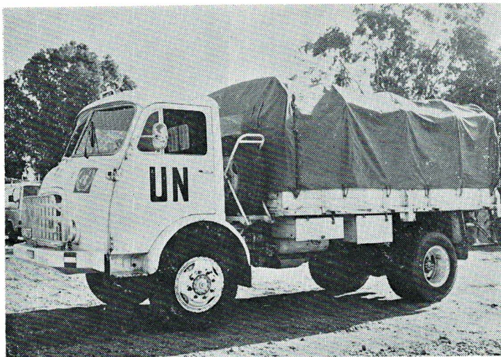
Steyer Diesel 680 (2-Achser): Payload 4500 kg; own weight 5430 kg; highest speed 80 km/h; 120 PS; hill-climbing-ability 58%.
