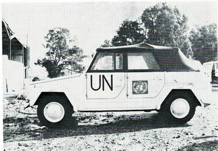
VW-181 (Hunter): Payload 440 kg; own weight 900 kg; highest speed 110 km/h; 48 PS; hill-climbing-ability 44%.
