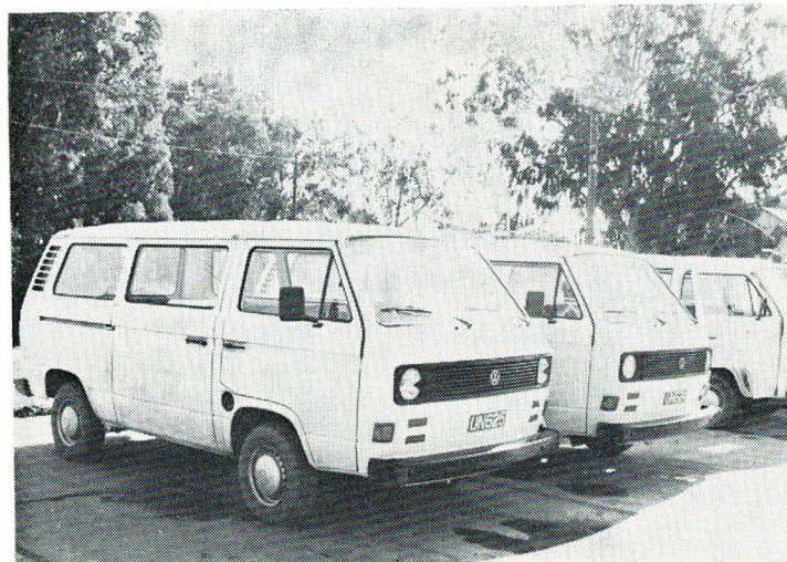
VW Bus: Payload 830 kg; own weight 1365 kg; highest speed 110 km, h; 50 PS; 9 persons including the driver.
